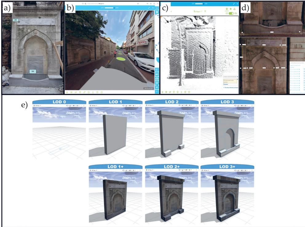
**Fig. 6.** İSKİ Fountain Information System Project data (a); IMM City Map Street Panorama Web Application screen (b); mobile lidar data accessed through Street Panorama application (c); measurement operations via Street Panorama application (d); 3D fountain model produced procedurally using designed data model (e)
