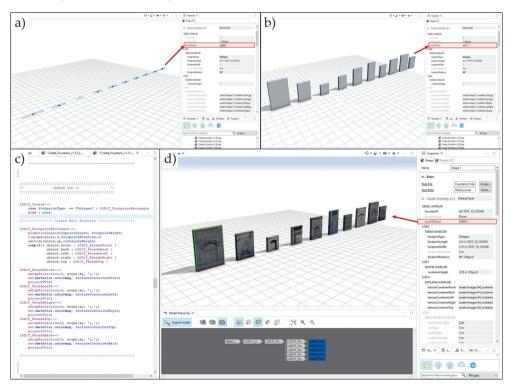
**Fig. 5.** Procedurally generated LOD0-level fountain footprints (a); procedurally generated LOD1-level solid model for fountains (b); procedurally algorithm for LOD1+ fountain models (c); procedurally produced LOD1+-level fountain models with facade textures (d)
