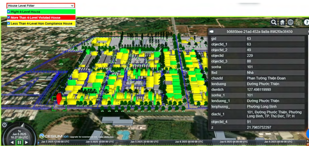
Fig. 15. Detect constructions violating height regulations
