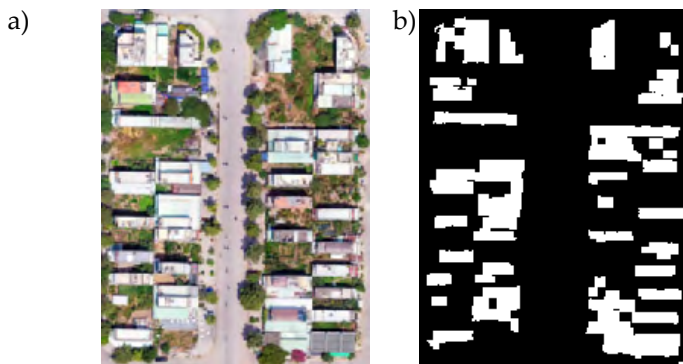
Fig. 7. Building footprint extraction results from DeepLabV3+ model: a) UAV imagery of buildings; b) predicted building footprints
